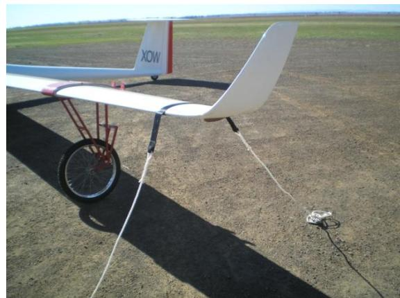
This tie-down strap has been made from rope and an old car seat belt to ensure nothing scratches the wing. Regular rope and large pegs over the tailboom will hold the tail down.
