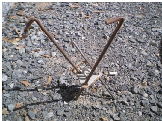
Ground stakes can be as simple as a large tent peg or a star picket but both suffer from either sticking out of the ground and puncturing car tyres and not being practical in different soils as well as being difficult to remove. The ground stake pictured is simple to make/safe if run over/works well in different soils by using different sized pegs and is easy to remove.
